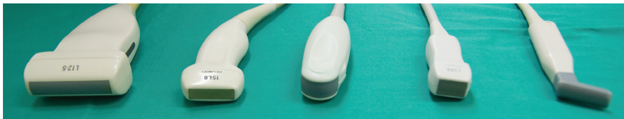
FIGURE 9.1 Ultrasound transducers for regional blocks. The photograph includes (left to right) broad linear, small footprint linear, curved, sector, and hockey stick transducers.
